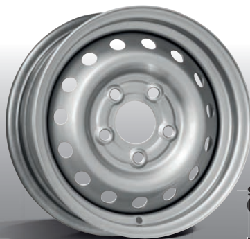
Stahlrad 0176 silver 5.0 x 13 load: up to 710kg
